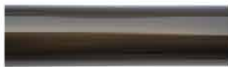
镜面阳极硬质氧化 HV700 Mirror surface hard anodize HV700 茶色 Dark brown
