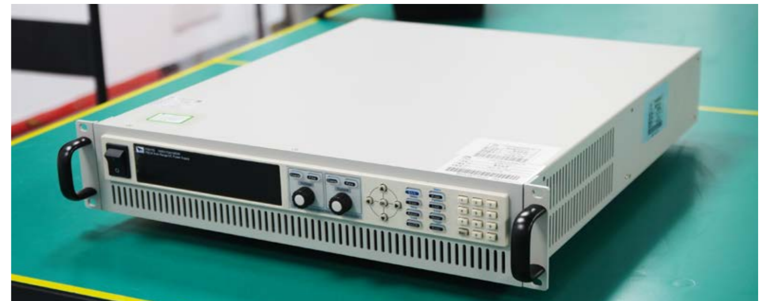
· 高电压直流稳定电源 High-voltage DC stabilized power supply
