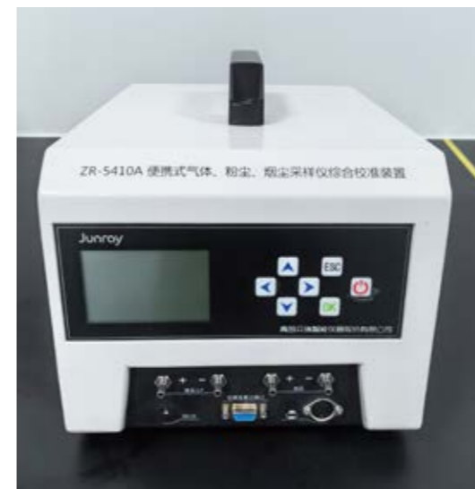
· 便携式气体、粉尘、烟尘采样仪综合校准装置： Portable gas, dust, smoke sampler comprehensive calibration device
