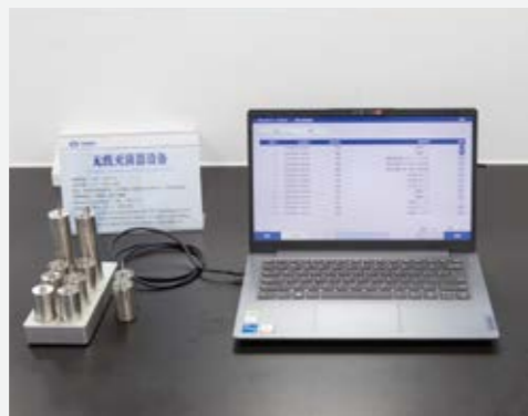
· 蒸汽压力试验设备校准装置 Calibration device for vapour pressure test equipment
